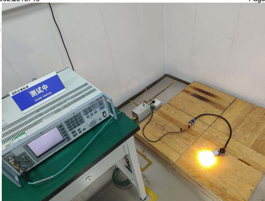
Continuous induced RF disturbances Test Setup-1
