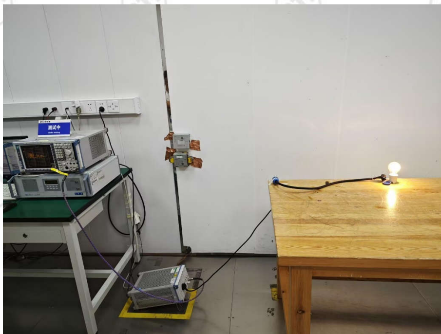
Conducted emissions Test Setup-1
