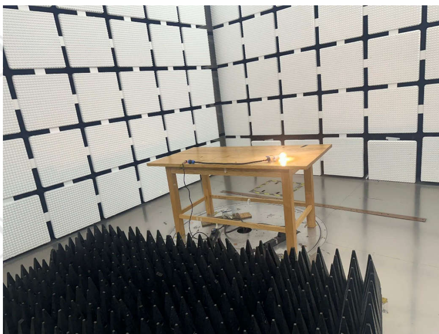
Continuous RF electromagnetic radiated field disturbances Test Setup-1
